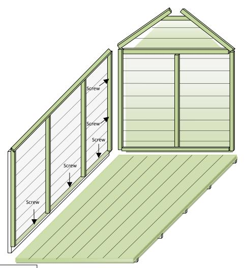
Stand the side panel with the 20mm overhang at bottom & flush with front of base.
