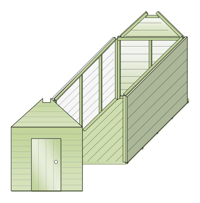
Fit the front panel and fix with 4mm x 70mm screws (same as sides & back)
