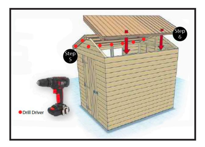
Once the roof is attached proceed to felt, starting at the lowest end working up to the highest end. Make sure the felt pieces overlap each other by at least 6" and the edges by 2".
